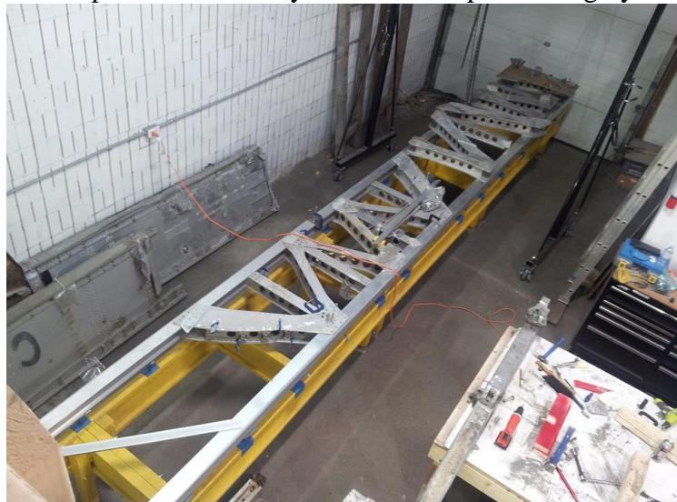
Main Spar final assembly with REAR spar waiting by wall
